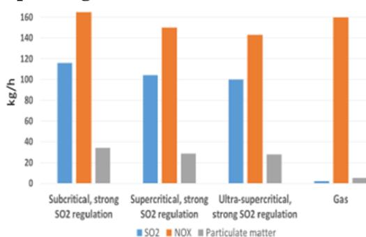
Figure 3: Air pollutant emission (coal and gas fired power plants).
