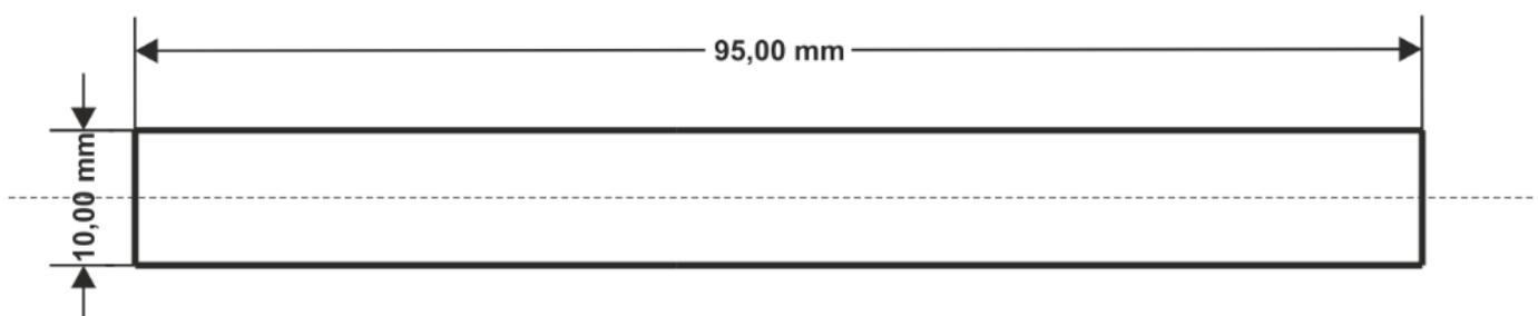
Figure 2: Specimen geometry for thermo-physical simulation experiments using the Gleeble system.
