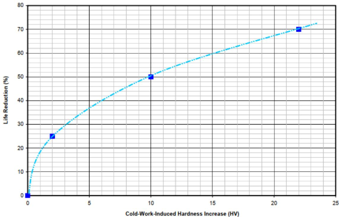
Figure 1: Creep life reduction as a function of hardness increase induced by cold-working.
