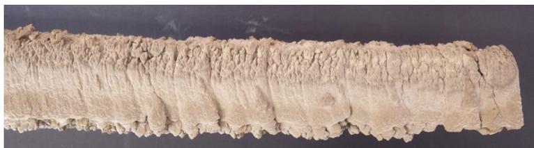
Figure 1: Superheater probe specimen string post exposure
