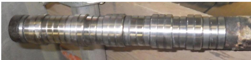
Figure 2: Corrosion probe with coupons prior to installation and exposure in operational boiler.
